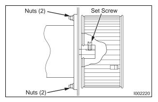
**3)** Loosen the set screw using a hex key. Then remove the fan motor by loosening four (4) nuts.
