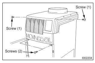
2) Remove four (4) screws from upper front panel.
