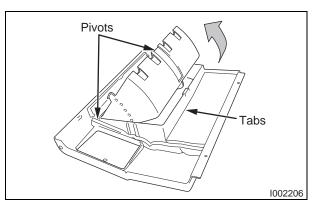
**4)** Louver can be removed from upper front panel by unsnapping the lock tap and removing the louver from its pivots.
