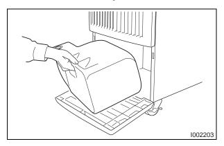
1) Remove drain tank.
