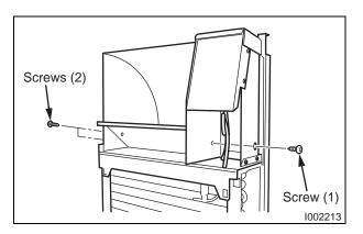
1) Remove three (3) screws from air deflector.
