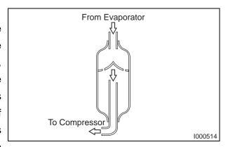
of gravity, causing the refrigerant to accumulate at the bottom of the vessel. As a result, the compressor is protected from possible damage caused by liquid refrigerant intake.
