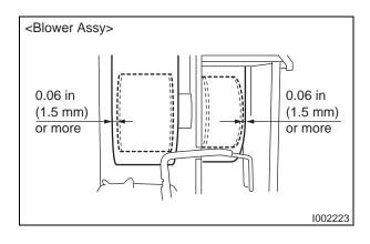
Install blower fan for evaporator and blower fan for condenser. Allow a clearance of 0.06 in (1.5 mm) or more on each side of the evaporator fan and the condenser fan.
