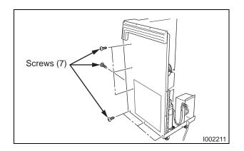
9) Remove seven (7) screws from right panel.
