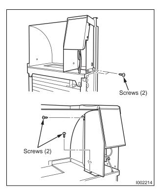
**2)** Remove four (4) screws from the control panel stay.
