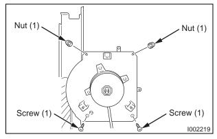
**2)** Remove two (2) nuts and two (2) screws as shown. Then remove the motor stay together with the fan motor.
