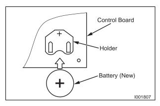
3) Insert new battery securely in the direction shown in the drawing.
