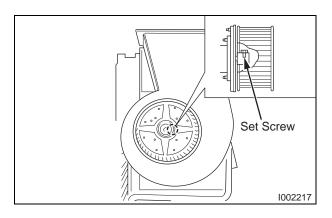
1) Loosen the set screw using a hex key. Then remove condenser fan.
