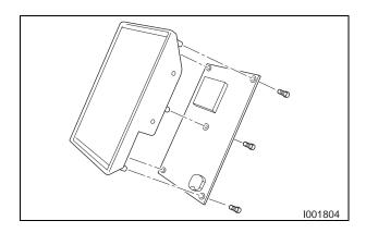
**4)** Remove the five (5) screws from the control board on the control panel assembly. Remove the control board.
