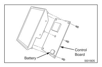
1) Disassemble control board. (See page 46 to 48.)
