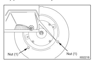
1) Remove two (2) nuts on the inside of the condenser fan casing in the locations shown. Then remove condenser fan casing.
