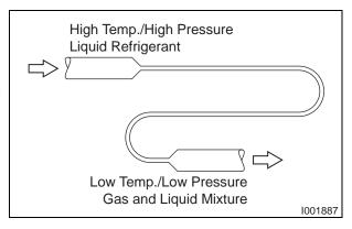
is sprayed out through the fixed orifice in the capillary tube. As a result, the temperature and state of the refrigerant becomes low and mist-like respectively, causing it to evaporate easily.
