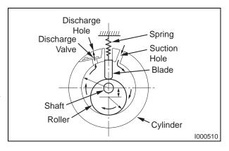
and the discharge side to keep compressed refrigerant from returning to the suction side. There is no suction valve. The discharge valve is designed not to open until the pressure of the refrigerant within the cylinder reaches or exceeds discharge side pressure. As a result, the discharge valve prevents the backward flow of refrigerant gas.
