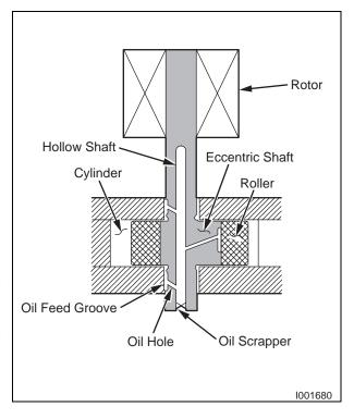
shaft journal keeps the bearing from being damaged during high temperature operation.
