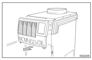
3) Slide upper front panel forward and remove.
